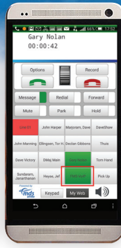
▲ Toggle key to move between GSM and VoIP, for a call in progress
